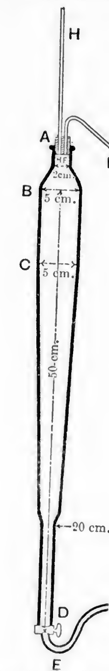
Fig. 40.—Schöne's Apparatus for Silt Analysis, Modified by Mayer.
